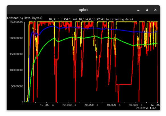
This is a much busier chart. BBR does not react to packet losses in the same way Cubic does. It is going to look at the changes in round-trip-time and achieved throughput when deciding on a congestion window. You can see that for this run, by and large the Red line remained
