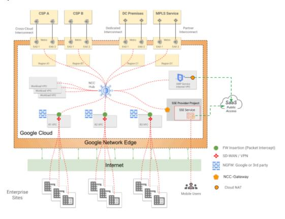
Site traffic aggregated using VPNs such as SD-WAN tunnels can be secured using a combination of cloud-native network security mechanisms. Traffic aggregated by the SD-WAN headends can be
