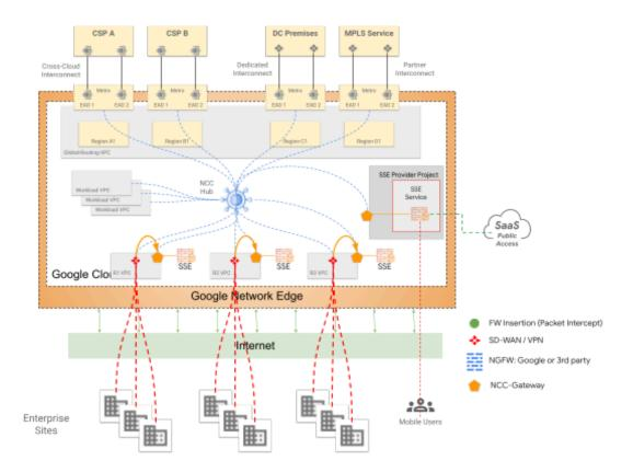
This pattern allows all site user flows to be secured via SSE. The following flows will be sent to the SSE service and then to their destination:
