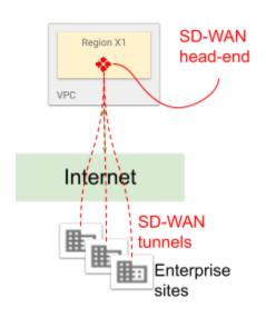
Site access aggregation: Sites will connect over the internet using an SD-WAN VPN to maintain privacy and enable the use of private address space. Google Cloud is ubiquitously connected to the internet in over 202 global peering points and offers highly reliable peering connections through its Validated Peering Partner program.
