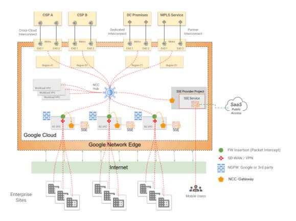
Internet bound site traffic aggregated using SD-WAN tunnels can be steered to an SSE service using private connectivity via the NCC Gateway. This is a high performance connectivity channel for traffic on-ramp to SSE services hosted in Google Cloud. The figure below depicts the design in which internet access to public SaaS is secured using an SSE stack. The following security surfaces are at play in this design:
