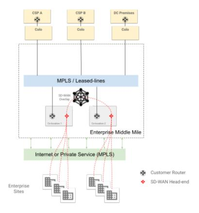
The existing middle-mile network can connect to the Google network using Cloud Interconnect (Dedicated Interconnect and/or Partner Interconnect) with up to 99.99% reliability SLAs. The SD-WAN overlay deployed over the middle-mile can be expanded to include head-ends hosted in cloud regions. Adding head-ends in Google Cloud, as shown in the following figure, allows the enterprise to easily expand their geographic footprint to aggregate user sites without operationalizing new co-locations.
